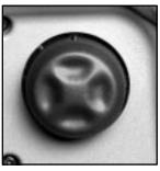
Use the lumbar control, located on the outboard side of the seat, to increase or decrease lumbar support in an area of the lower seatback.
